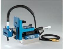
The new Slug Retention Machine uses a pneumatically-powered grinder to precisely machine a small angled groove into the sidewall of the die cavity in a stamping die. A micrometer coupled to the drive of the machine's slide enables precise movement of the machine's carriage to enable the depth of the slug retention groove to be precisely controlled
